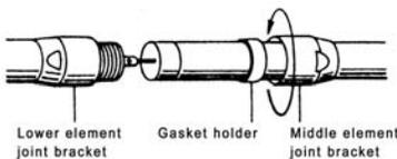
5. Fasten each connecting section firmly to have no gap between each shell with wrench.
