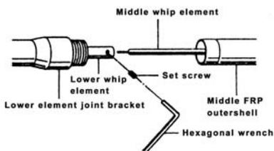
4. Put middle element shell into lower element shell until it reaches the gasket and fix them with joint element shell joint brackets.
