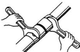
6. Attach three radial elements as shown in Fig. A.
