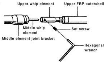
2. Put upper FRP element shell into lower FRP element shell until it reaches the gasket and fasten them with joint bracket.
